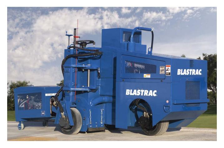
The Blastrac® BMP 6000 electric milling machine is designed for heavy surface preparation. Different milling cutter configurations allow this machine to remove concrete, overlayments, asphalt, troweled down epoxies, elastomeric coatings, thin-set mortar, grout beds, and flooring materials such as ceramic tile.
